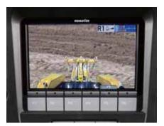
Fully integrated rear-view camera system
