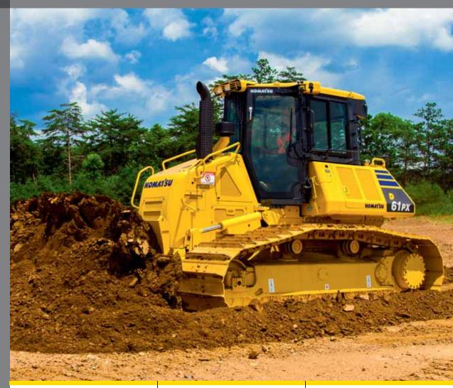
ENGINE POWER 126 kW / 169 HP @ 2.200 rpm **OPERATING WEIGHT** D61EX-24: 18.520 kg D61PX-24: 19.460 kg **BLADE CAPACITY** D61EX-24: 3,4 m<sup>3</sup> D61PX-24: 3,8 m<sup>3</sup>
